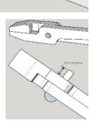
**Split Jaw** tongs are a variation that holds round and square stock very securely. The process for these is the same, except the jaws are not twisted.
